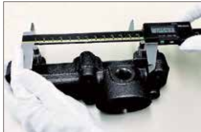
ノギスでねじ穴のピッチを測定 Center-to-center measurement with calipers
